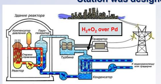
**Pressurized Water Reactor (PWR)**
