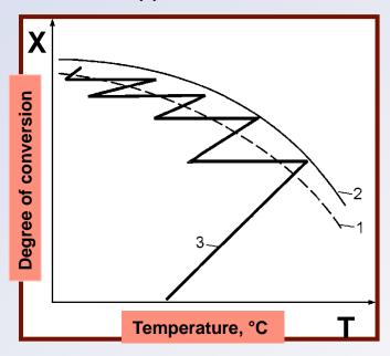
G.K. Boreskov, M.G. Slinko, Zh. Prikl. Khim 16 (9-10), 377, 1943. // Principles of the design of Contact Reactors for reversible exothermic reactions
