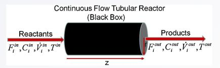
Also «M.G.» denoted the treating a reactor as a black box. The method of multiple-correlations to find a functional correlations between parameters at the inlet and outlet of a reactor were rejected, because they did not reflect the peculiarities of the process and could not serve as a basis for the scaling-up.
