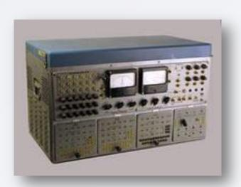
MN-7, a vacuum-tube analog computer, which could solve systems of nonlinear ordinary differential equations up to the sixth order.
