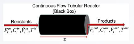
Also «M.G.» denoted the treating a reactor as a black box. The method of multiplecorrelations to find a functional correlations between parameters at the inlet and outlet of a reactor were rejected, because they did not reflect the peculiarities of the process and could not serve as a basis for the scaling-up.
