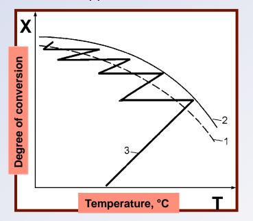
G.K. Boreskov, M.G. Slinko, Zh. Prikl. Khim 16 (9-10), 377, 1943. // Principles of the design of Contact Reactors for reversible exothermic reactions
