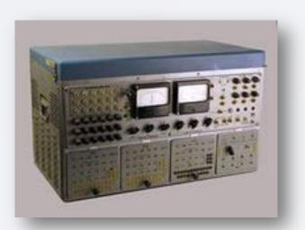
MN-7, a vacuum-tube analog computer, which could solve systems of nonlinear ordinary differential equations up to the sixth order.
